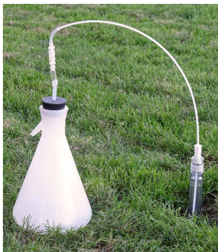
Fig. 12 - Connect the Sampler to the Erlenmeyer Flask.
