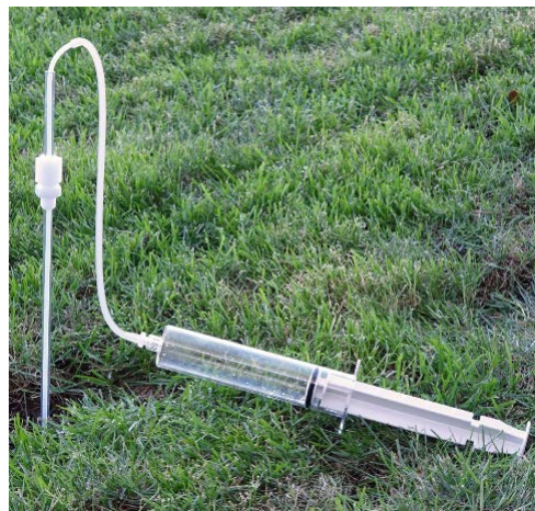
Fig. 11 - Syringe collecting a sample (NOTE: The Cloth Bag should be used for outdoor applications.)
