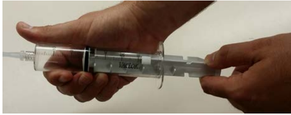
A. Connect Locking Syringe to 1909 sampler and then pull the Syringe Handle.
