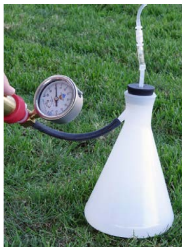
Fig. 13 - Apply 80 cb of vacuum using the Vacuum Hand Pump
