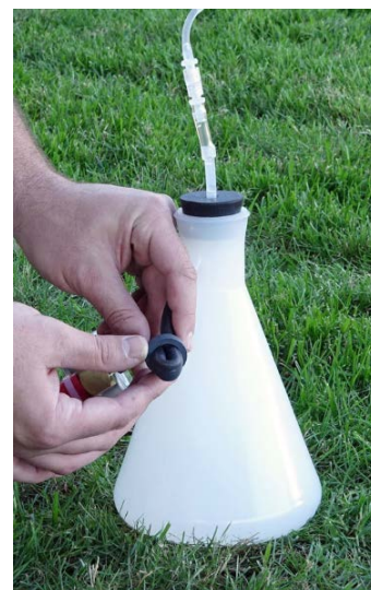
Fig. 13 - Close off the EPDM Tubing before disconnecting the Hand Pump
