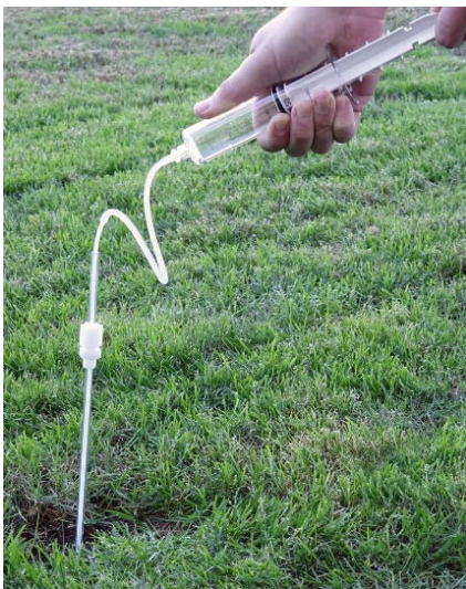
Fig. 10 - Pulling a vacuum with the 1930 Vacuum Syringe
