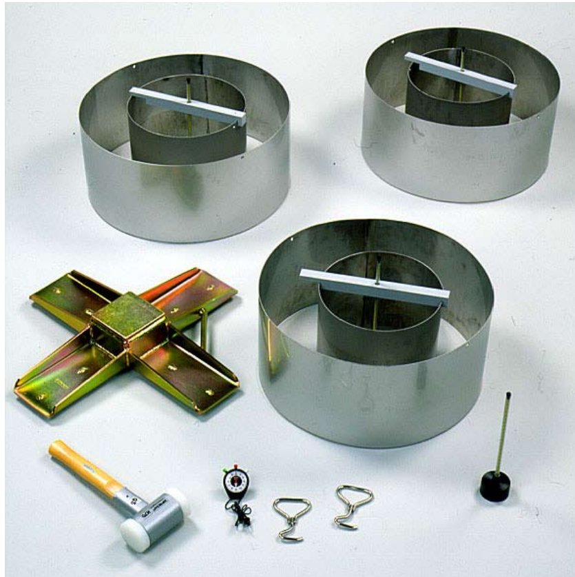
(Figure 1) - 2830K1 Double Ring Infiltrometer Kit
